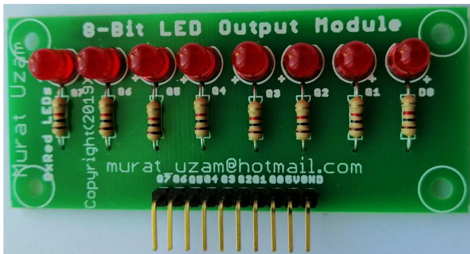
Top view (component side) of the soldered 8-Bit LED Output Module.
